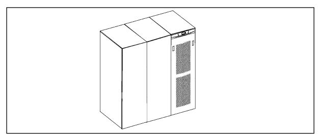
Figure 2 UPS configuration with two External Battery Cabinets.
